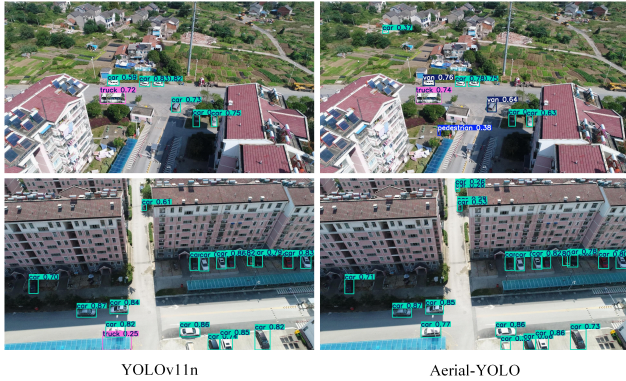
Fig. 6. Detection results of YOLOv11 and Aerial-YOLO under complex background conditions.
