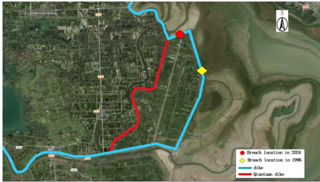
Fig. 7. Schematic Diagram of the Location of the Tuanzhou Embankment Breach (Modified based on the monitoring data of Hunan Water Conservancy Department [7]).
