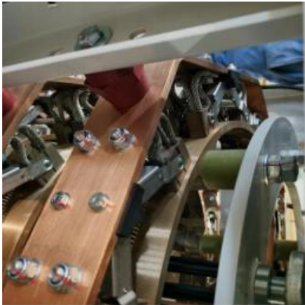
FIGURE 1. Actual Overall Slip Ring Structure
