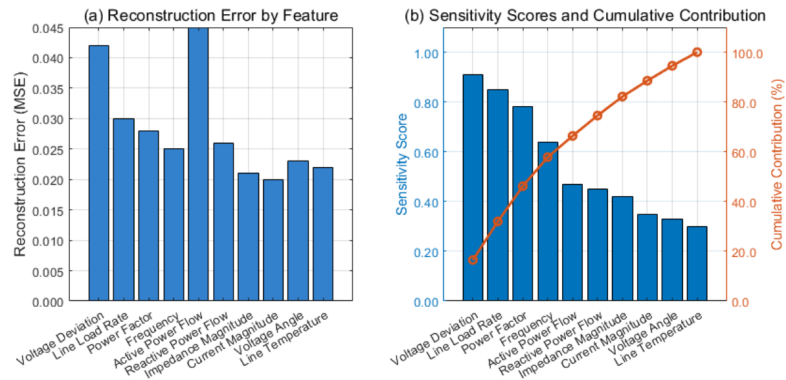
FIGURE 2. Importance of power grid features and reconstruction error under sparse autoencoder. Figure 2(a). Reconstruction Error Feature. Figure 2(b). Sensitivity Score and Cumulative Contribution
