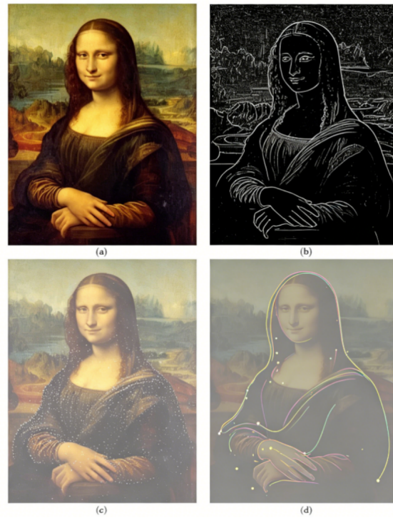
FIGURE 2. Flowchart of vectorized extraction of geometric features of brushstrokes. (a) Original digital art image. (b) Adaptive Canny edge detection results. (c) Edge feature point extraction. (d) Vectorized fitting results of Bézier curves
