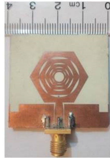
FIGURE 6. Fabricated prototype of the proposed CPW-fed slotted hexagonal antenna.
