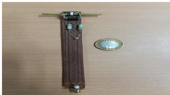
FIGURE 2. developed design of fabricated Electric field probe.
