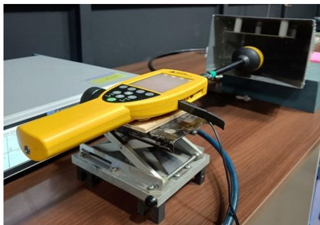
FIGURE 7. Calibration and measurement setup of E-field (a) developed probe (b) standard reference probe NBM-50.
