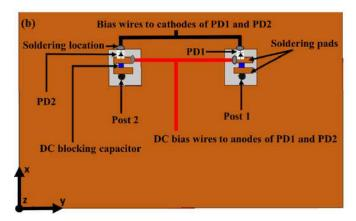
FIGURE 2. (a) Top, and (b) Bottom view of initial antenna geometry.
