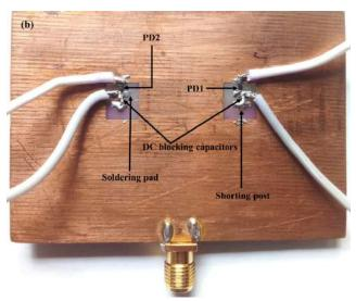
FIGURE 6. Fabricated antenna (a) Top, (b) Back side.
