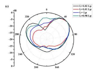
**FIGURE 5.** (a)  $S_{11}$ , (b) E plane, and (c) H plane radiation pattern, for different values of L.
