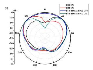
**FIGURE 3.** (a) Reflection coefficient, (b) E plane, and (c) H plane radiation pattern of initial antenna geometry for different modes.
