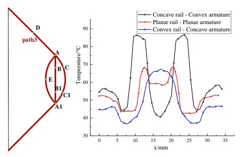
FIGURE 11. Schematic diagram of path 3 and temperature distribution
