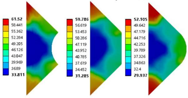
FIGURE 10. Cross-sectional view of temperature distribution at the end of the rail for different configurations
