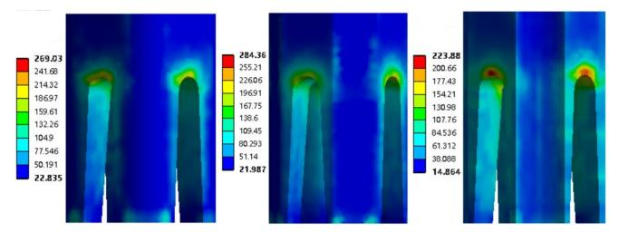
FIGURE 7. Schematic diagram of armature temperature distribution of different configurations
