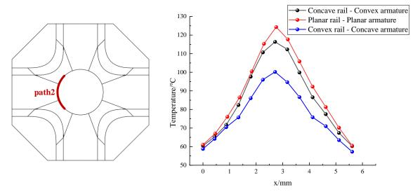
FIGURE 9. Schematic diagram of path 2 and temperature distribution
