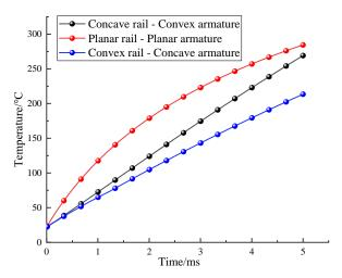
FIGURE 6. Schematic diagram of the maximum temperature variation of electromagnetic launchers of different structures
