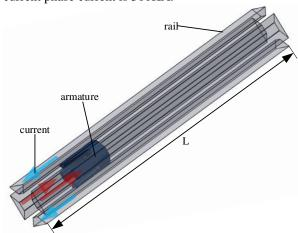
FIGURE 1. Four-rail electromagnetic launcher model
