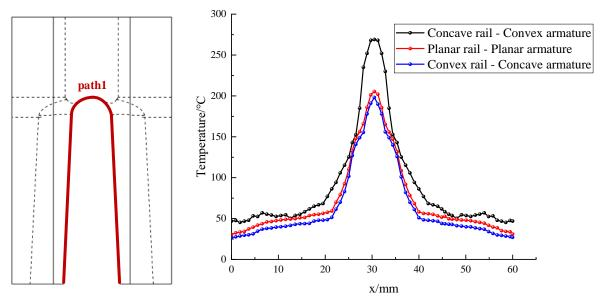
FIGURE 8. Schematic diagram of path 1 and temperature distribution
