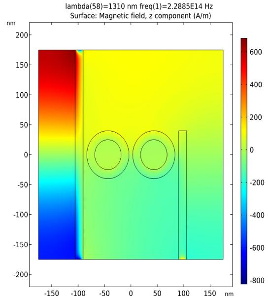
Figure 2: The Magnetic Field Profile in Case of (ON) Output State.
