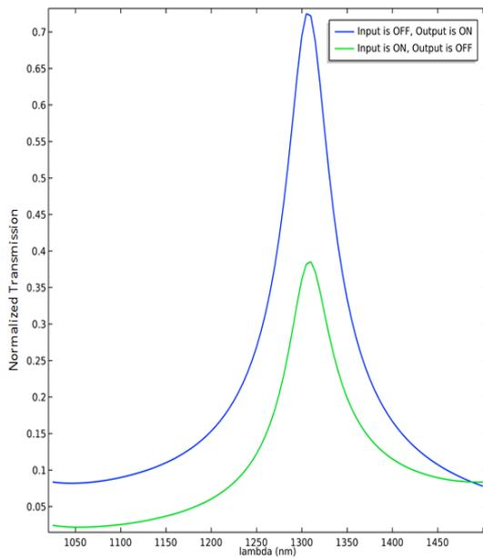
Figure 4: Optical Transmission as a Function of Wavelength at the Different Condition States.
