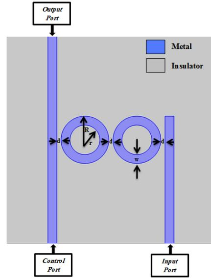
Figure 1: The Proposed Structure of All-Optical Plasmonic NOT Gate.
