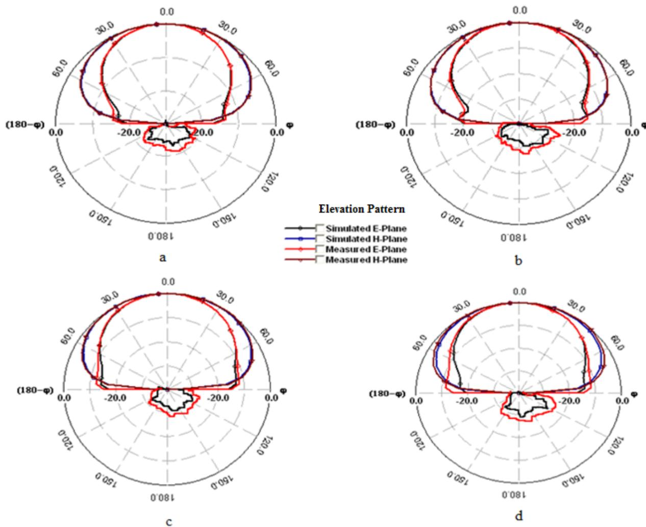
Figure 6. Simulated and measured E-plane and H-plane radiation patterns at: a-1GHz, b-1.5GHz, c- 2GHz, d-2.5GHz
