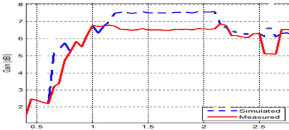
Figure 4. The simulated and measured gain of proposed antenna
