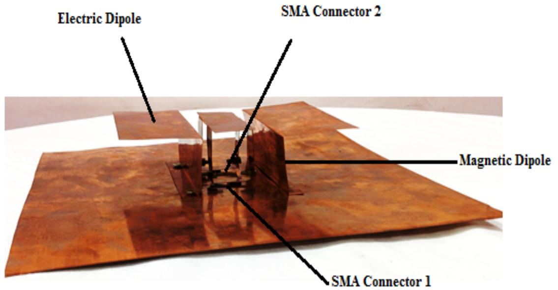
Figure 1a. Prototype of proposed antenna with side view of feed
