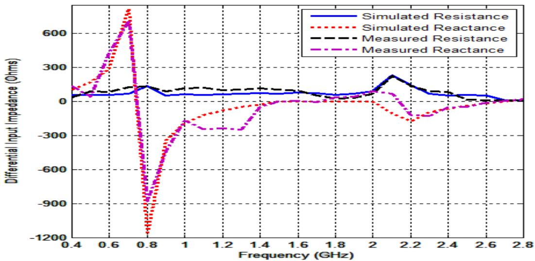
Figure 5. The simulated and measured differential input impedance
