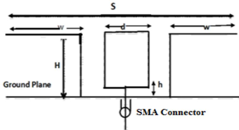
Figure 2a. Side view of the proposed antenna
