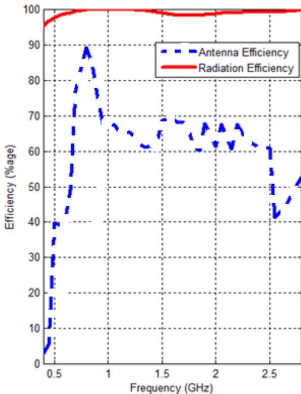
**Figure 7. Simulated antenna efficiency and radiation efficiency of proposed antenna**
