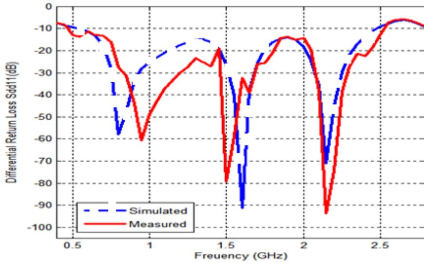
Figure 3. The simulated and measured differential return loss,  $S_{dd11}$
