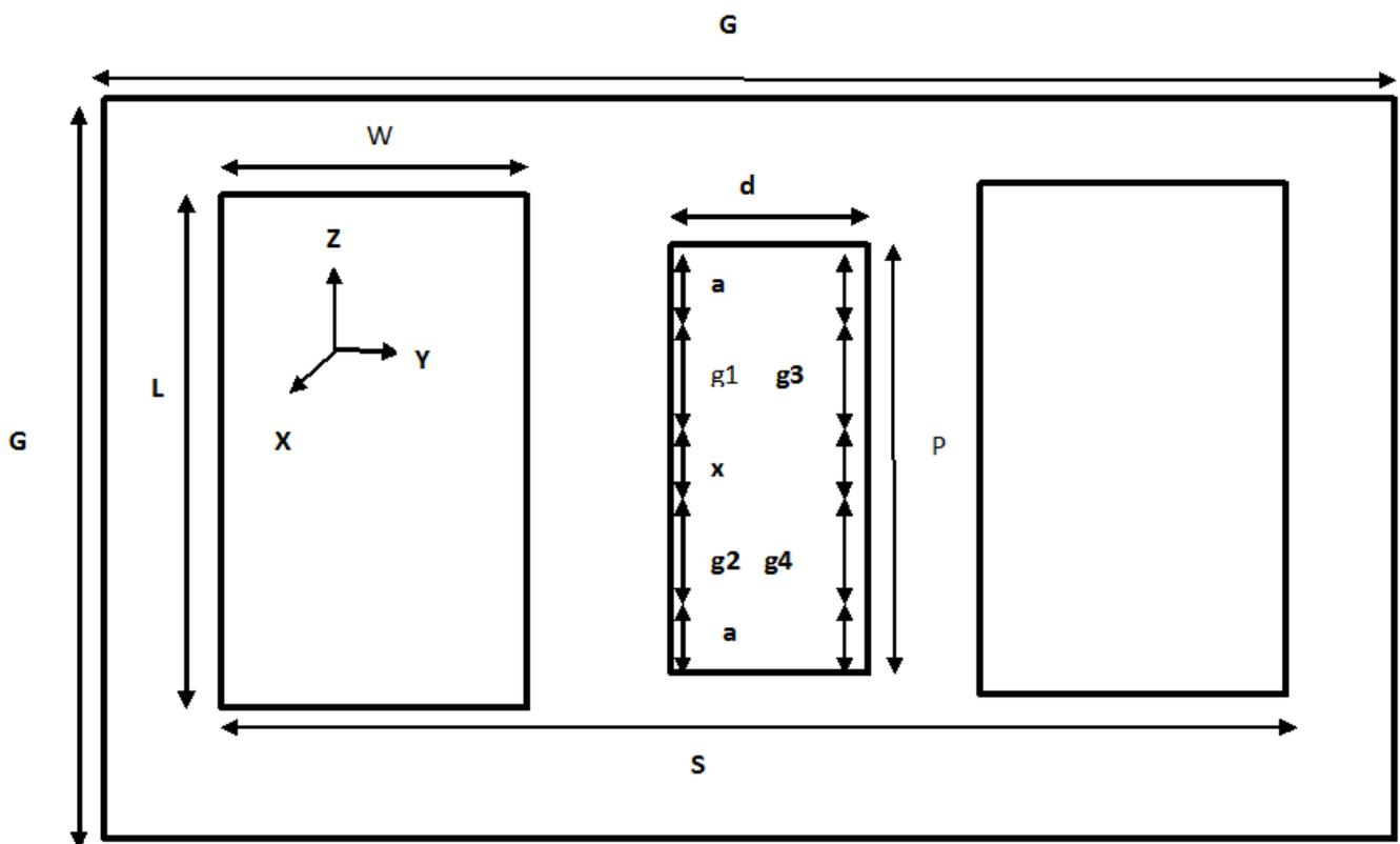
Figure 2b. Top view of the proposed antenna
