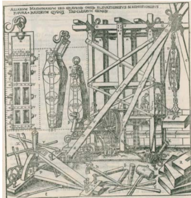
FIGURE 3. Reconstruction drawings of ancient Roma cranes from liber X of Vitruviusby
