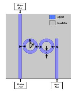
Figure 1: The Proposed Structure of All-Optical Plasmonic NOT Gate.
