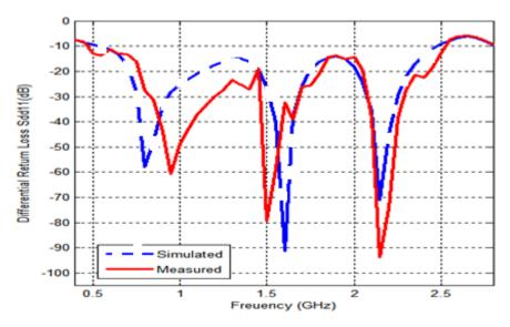
Figure 3. The simulated and measured differential return loss,  $\mathbf{S}_{dd11}$
